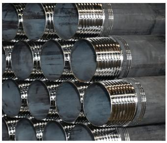
Di-Corp drill rods come with engraved indicator grooves on the outside of the rod to quickly identify the thread. One groove for R thread, two grooves for D thread, three grooves for S-Maxx (pictured), and no grooves for standard wireline.
