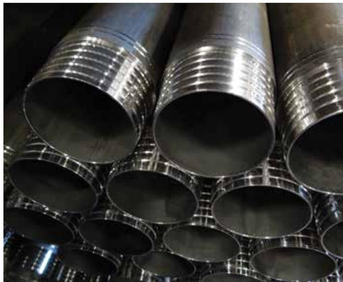
Di-Corp drill rods come with engraved indicator grooves on the outside of the rod to quickly identify the thread. One groove for R thread, two grooves for D thread (pictured), and no grooves for standard wireline.
