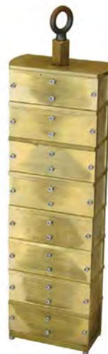
#122-085 - 16 Specimen Cement Mold Assembly
