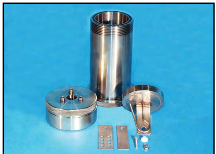
#175-40 - Corrosion Test Cell
