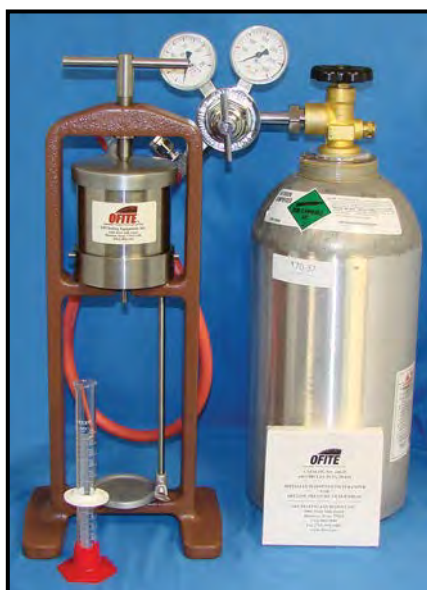
#140-35 - Filter Press with Nitrogen Pressurization
