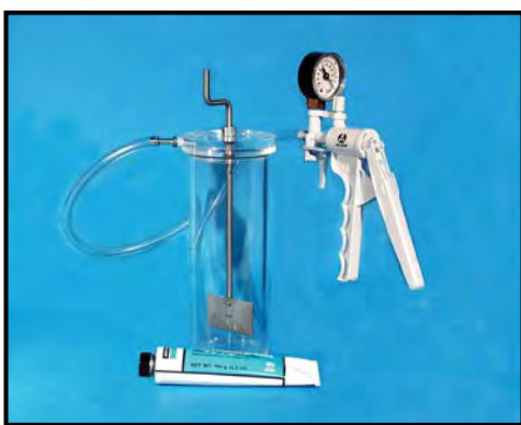
#110-00 - Mud Deaerator with Vacuum Pump
